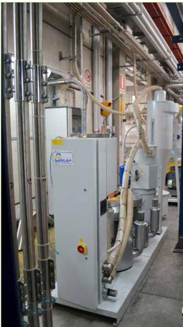
The typical solution of a pneumatic conveying system foresees: one vacuum blower, in most cases there is one backup pump in stand-by, and one main filter with automatic cleaning. A pneumatic by-pass valve on the vacuum blower allows motor continuous operation. Pipe cleaning valves are suitable to purge pipe lines from material maintaining the lines free from stagnant material avoiding from risks of overloads for pipe clogging, discontinuous feeding and cooling of dehumidified materials.
